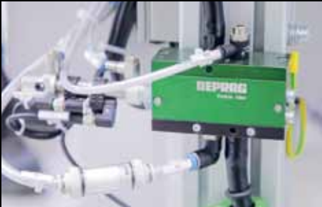
DEPRAG particle killer: dirt particles are targeted and removed from the conveyor
